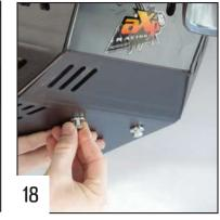
Put the alloy spacers in the front holes, then place 2 TH 6x40mm screws without tightening.
