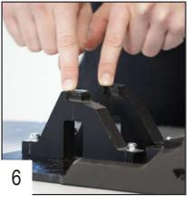
Place the 2 rear fixations in plastic using 4 TFHC 6x30mm screws. The machined sides must be on the right.
