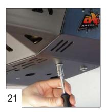
Tighten all the screws, starting with the rear screws, then the middle and the front.
