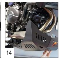
Place the skid plate under the frame.
