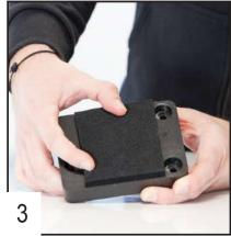
Stick the foam on each side of the skid plate and on the plastic block.
