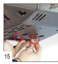
Place 2 TFHC 6x35mm screws in the middle holes to keep the plate in place, do not tighten.
