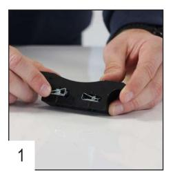
Place the clamped bolts in the front fixation.
