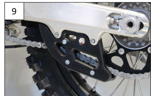
8 Place the second bloc, clip it and tight with the Tfhc 6x60mm screws, M6 Washers and em6f
