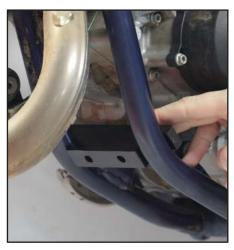
Place the front fixation in the frame and clip it inside the bars.
