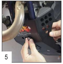
Lift the skid plate up to put the THF 6x25mm screw in.
