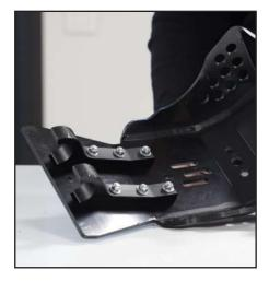
Place the 2 plastic hooks on the rear of the skid plate using TFHC 6x30mm screws + M6 washers and EM6F bolts, then tighten.
