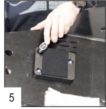
Place the plastic block on the bottom of the skid plate using 3 TFHC 6x25mm screws + M6 washers and bolts then tighten.
