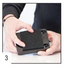
Stick the foam on each side of the skid plate and on the plastic block.
