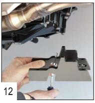
Use 2 TCHC 6x30mm screws + M6 washers to fix the front fixation directly on the engine block and tighten.
