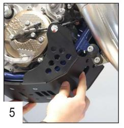
Lift the skid plate up to put the special screws in.
