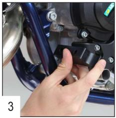
Place the front fixation in the frame and clip it inside the bars.
