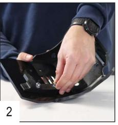
Place the 2 plastic hooks on the rear of the skid plate using TFHC 6x25mm screws + M6 washers and EM6F bolts, then tighten.
