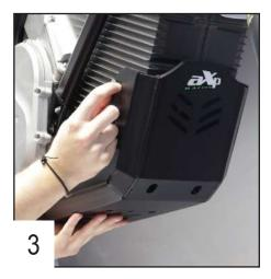
Place one TFHC 8x20mm screw on each side without tightening.
