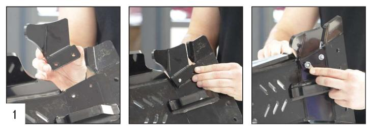
Place the footpeg protection on the right side using 2 TFHC 6x25mm screws + M6 washers and bolts, then tighten.
