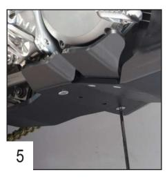
Tighten the rear screws.
