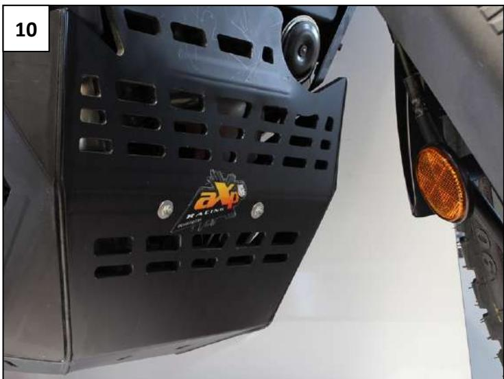
**Fit the two front screws at the front to finish the assembling**
