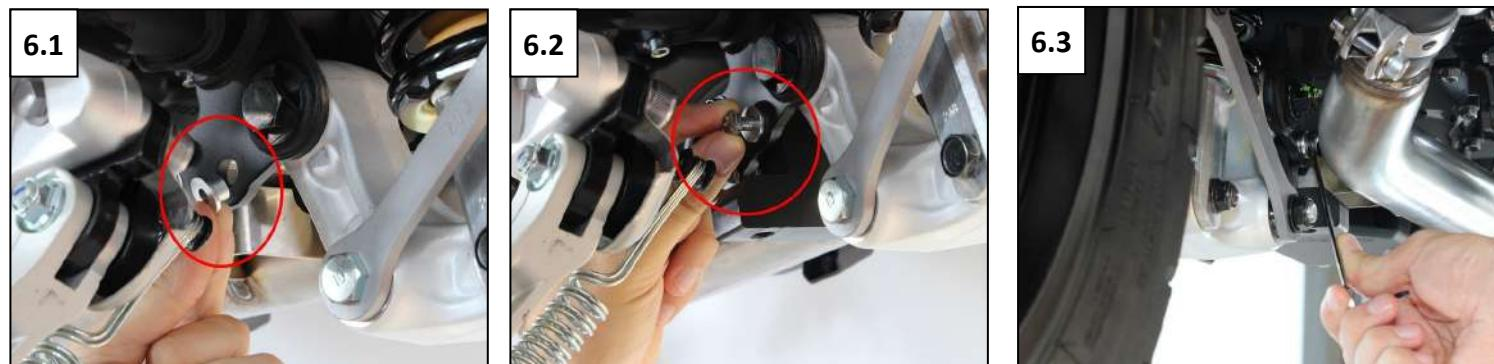
**Put the 2 alloys spacers on each side of the frame support (6.1) , place the plastic mount and pass the Th 6x70mm screw through (6.2). Add the bolt on the right side of the frame support and tight everything (6.3)**
