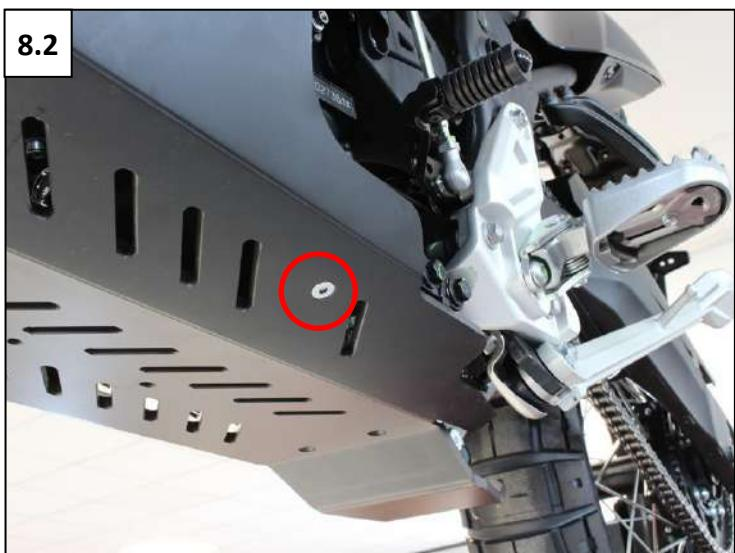
**Put the skid plate in place by fixing the 2 Tfhc 6x25mm on each side and tightening it.**
