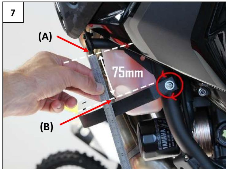
**Before putting the skid plate in place, adjust the front fixation by rotating it. You have to set a distance of 75mm between the frame tube bottom (A) and the top surface of the plastic bracket (B). Then the plastic mount holes and the skid plate holes will be aligned**
