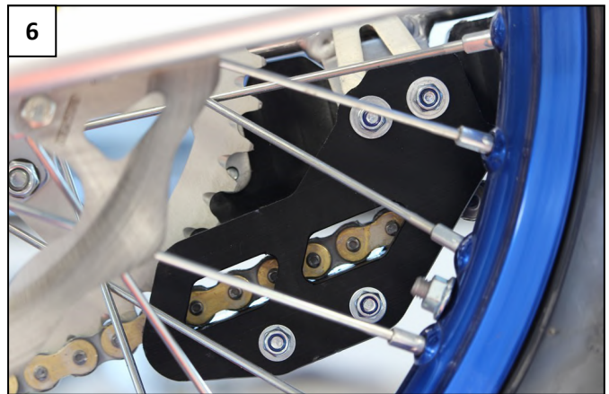
6 Place the em6f + M6 Washers and tight it Placer les em6f + M6 washers et serrer
