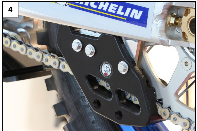
4 Place the Th 6x60mm + Th 6x15mm Placer les Th 6x60mm + Th 6x15mm
