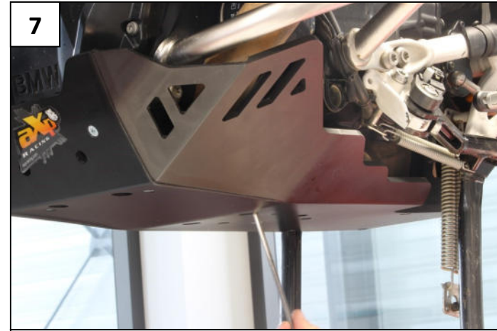
7 Place the 3 Tbhc 8x50mm screws in the middle of the skid plate with M8 Washers and tight everything
