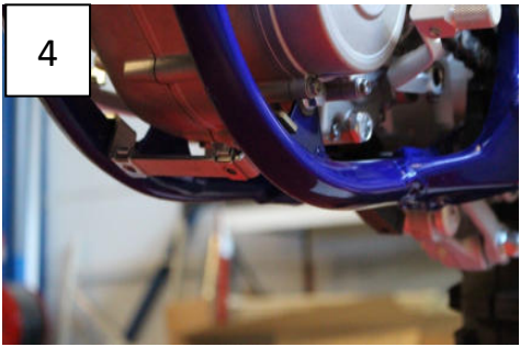
Install PM02-01-031 and fit the front of the skid plate
