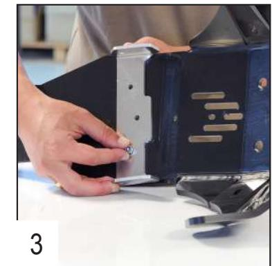
Use 2 TFHC 6x20mm screws + M6 washers and bolts to fix the aluminum part without tightening.
