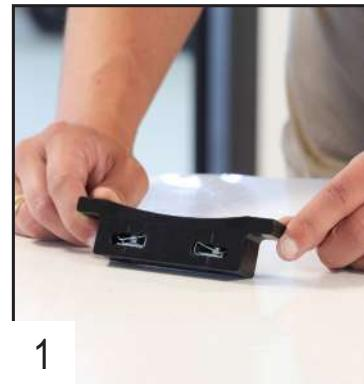
Insert the clamped bolts in the front fixation.
