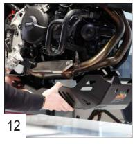
Place the skid plate under the frame.
