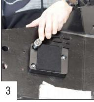
Place the plastic block on the bottom of the skid plate using 3 TFHC 6x25mm screws + M6 washers and bolts then tighten.
