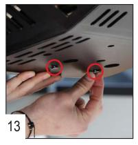
Place 2 TFHC 6x35mm screws in the middle holes to keep the plate in place, do not tighten.
