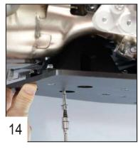
Place 2 TCHC 6x45mm screws + M6 washers in the rear fixations without tightening.
