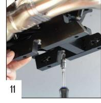
Use 2 TCHC 6x30mm screws + M6 washers to fix the front fixation directly on the engine block and tighten.
