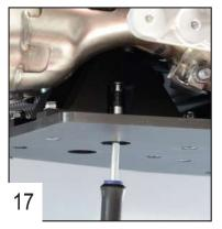
Tighten the rear screws.
