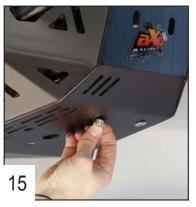
Put the alloy spacers in the front holes, then place 2 TH 6x40mm screws without tightening.
