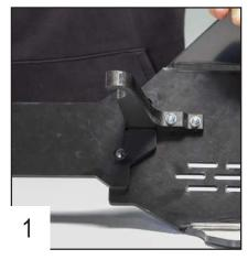
Insert the linkage guard at the rear of the plate.
