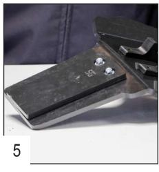
Use 2 TFHC 6x20mm screws + M6 washers and bolts to fix the linkage guard on the plate.
