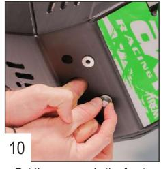
Put the spacers in the front holes and use 2 TH 6x30mm screws to fix the plate. Use the bigger hole to maintain the fixation in place with your finger.
