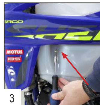
3 Remove the side screws to have a better access to the radiators.
