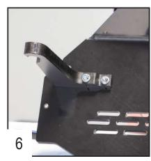
Place the rear bracket, make sure to use a TFHC 6x30mm screw in the longest hole and a TFHC 6x25mm screw in the smaller one.
