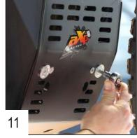
Tighten the rear and then the front screws.
