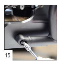
Insert the crash bars in the holes and use the OEM screw to fix the bar and the skid plate together to the frame.
