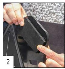
Cut the foam in two pieces and stick one on each side of the skid plate.
