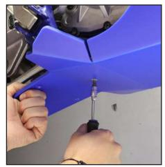
Place the TFHC 6x25mm screw in the rear hole. Then tighten.
