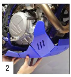
Place the skid plate under the frame to align the holes with the clamped bolts.
