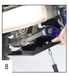
Fix the plate using 2 TFHC 6x20mm screws + M6 washers and bolts.
