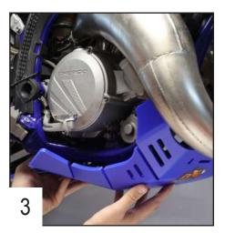
Clip the plate on the frame using the two rear hooks.
