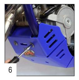
Place 2 THF 6x25mm screws in the front holes and tighten.
