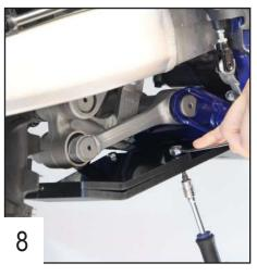
Fix the plate using 2 TFHC 6x20mm screws + M6 washers and bolts.
