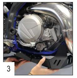
Clip the plate on the frame using the two rear hooks.
