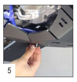
Place a TFHC 6x25mm screw in the rear hole.
