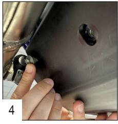
Place 2 THF 6x25mm screws in the front holes and tighten.
