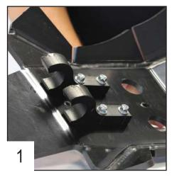
Fix the rear hooks on the skid plate using TFHC 6x30mm screws + washers and bolts and tighten.
