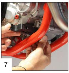
Place the front fixation in the frame and clip it.
