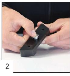
Place the alloy spacer in the rear fixation.
