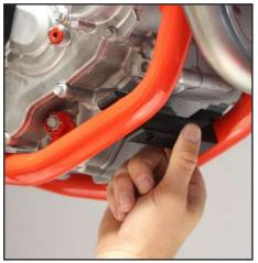
Place the skid plate and use a TH 6x30mm screw in the rear hole to maintain it, then tighten.
