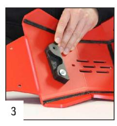
Fix the rear fixation using 2 TFHC 6x35mm screws + large washers and bolts.
