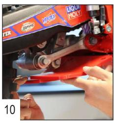
Pull the plate down to place the linkage guard.
