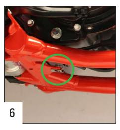
Place the clamped bolt directly on the frame, the flat side facing down.
