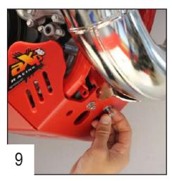
Place 2 TH 6x30mm screws in the front holes, then tighten. You can use the bigger hole to place the fixation correctly.
