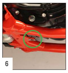
Place the clamped bolt directly on the frame, the flat side facing down.
