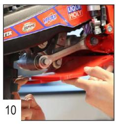
Pull the plate down to place the linkage guard.
