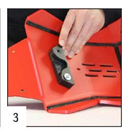
Fix the rear fixation using 2 TFHC 6x35mm screws + large washers and bolts.
