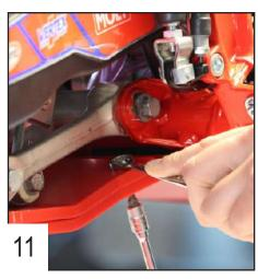
Fix the guard with 2 TFHC 6x20mm screws + washers and bolts.
