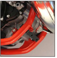
Place the skid plate and use a TH 6x30mm screw in the rear hole to maintain it, then tighten.
