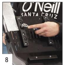
Use 6 TFHC 6x25mm screws + M6 washers and bolts, then tighten. Make sure to put the screws in the small machined holes.
