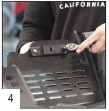
Tighten and make sure to place the longer machined part on the left.
