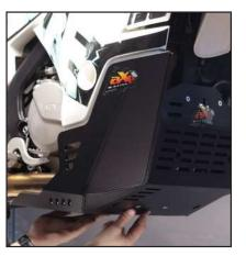
Place the skid plate under the frame. The machined faces must be perfectly aligned with the holes on the frame.
