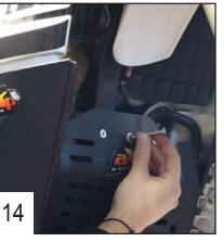
Place the TH 6x45mm screw to fix the front part of the plate.
