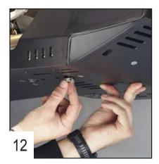
Place 4 TH 6x30mm screws + large M6 washers under the plate without tightening.
