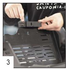
Cut the foam pads and stick them on each side of the plate to protect the tank.
