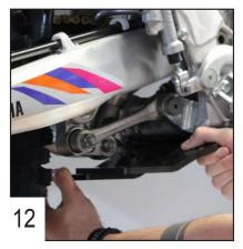
Push the plate down and place the smaller plate under the linkage.
