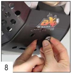
Use your finger to maintain the plastic block in place and put the 2 special screws.
