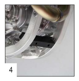
The HDPE plastic block must be clipped in the middle of the frame.
