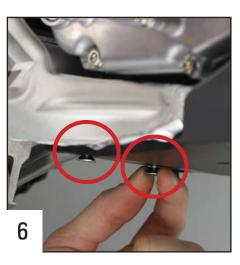
Place the 2 TFHC 6x16mm screws in the rear holes.
