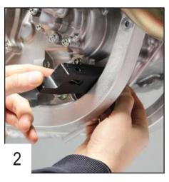
Place the HDPE plastic block inside of the frame.
