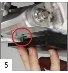
Put the plate in position and use the hole at the bottom of the frame to fix the rear end.
