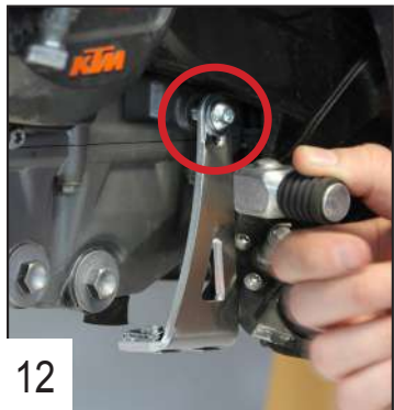
12 Place the smaller alloy part in place on the left side using the TBHC 8x20mm screw + M8 washer. Do not tighten.
