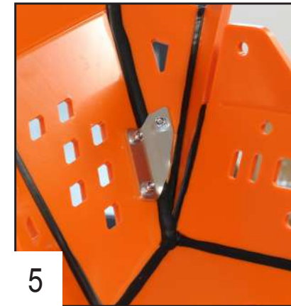
4 Fix the alloy parts on each side of the skid plate using 3 TFHC 6x20mm screws + M6 washers and EM6F bolts.
