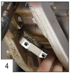
Place the front steel fixation in the frame. The insertion can be tricky, make sure to place the left side first.
