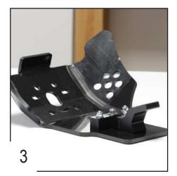
Place the rear fixation on the skid plate and fix it using the TFHC 6x35mm screws + EM6F bolts and M6 washers.
