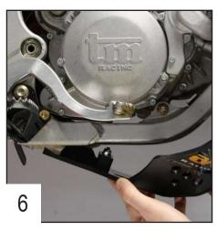
Clip the hook on the frame and lift the skid plate to put it in the correct position.
