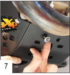
Put the first special screw in the front hole. Use the big hole to maintain the fixation in place.
