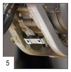
The fixation must rest on the welds.
