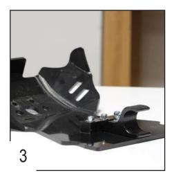
Place the rear fixation on the skid plate and fix it using the TFHC 6x30mm screws + EM6F bolts and M6 washers.
