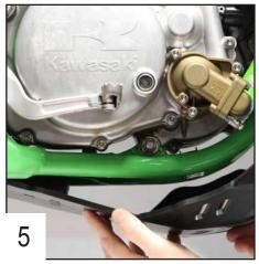
Clip the hook on the frame and lift the skid plate to put it in the correct position.
