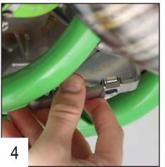
Place the front steel fixation in the frame.
