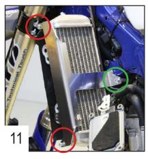
Place the rear part using the TFHC 6x16mm screw in the right hole and two TBHC 6x16mm screws in the top and bottom holes, without tightening.
