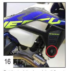
Put the tank back and don't forget to tighten the screw. Then, put the plastics back in place and use one TBHC 6x30mm screw + M6 washer on each side to fix it.
