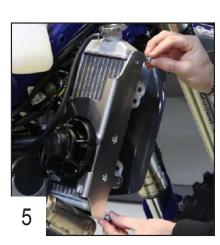
Place 2 TBHC 6x16mm screws in the top and bottom holes to fix the 2 parts together without tightening.
