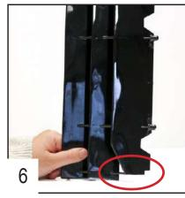
Cut the bottom of the air deflectors for a perfect fitment with the guards. You must cut the closest parts from the frame.
