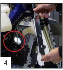
Put the rear side in place. Make sure to pass the guard under the wires.
