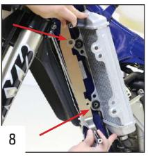
Place the front guard on the other side, and fix it with the two OEM screws.
