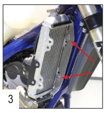
Remove the plastics, the tank and the two OEM screws. Then place the front side and use the OEM screws to fix it.
