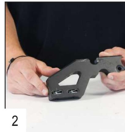
2 Place 2 clamped bolts in each front fixation.
