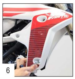
Place the plastic protection back in place and use the TBHC 6x25mm + M6 washer in the bottom hole.
