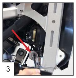
Place the aluminium guard on the radiator using the OEM screw.
