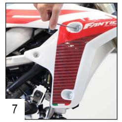
Place the TBHC 6x25mm screw + M6 washer in the top hole.
