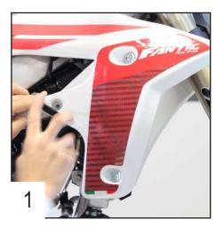
Remove the plastic protections on both sides.
