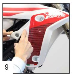
Use the 6x20mm screw + M6 washer and tighten all the screws. Then, repeat the operation on the other side.
