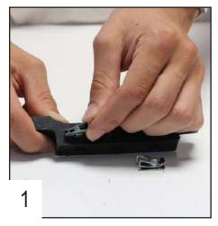
Place two clamped bolts in the 20mm front plastic part.
