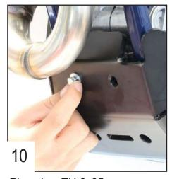
Place two TH 6x35mm screws + M6 washers in the front holes.
