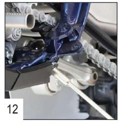
Tighten the screws on both sides.
