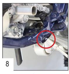
Remove the OEM screws on both sides.
