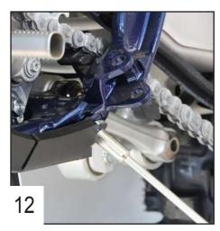
Tighten the screws on both sides.
