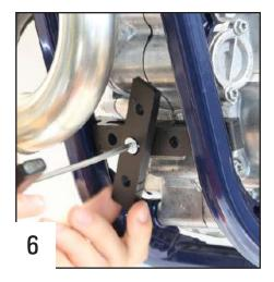
Use the 8mm plastic part and a TFHC 6x16mm screw to fix it on the frame.
