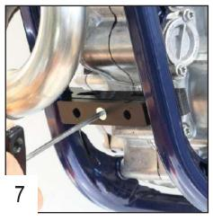
Adjust it in height so it rests on the welds of the frame and tighten the screw.
