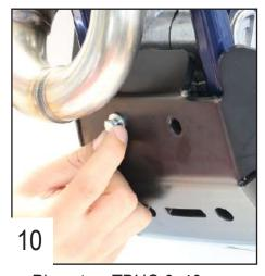
Place two TBHC 6x40mm screws + M6 washers in the front holes.
