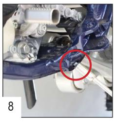
Remove the OEM screws on both sides.
