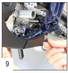
Place the plate on the bike and put the OEM screws back in place without tightening.
