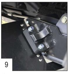
Choose the height and use the TBHC 8x40mm screws + bolts and washers to fix it.
