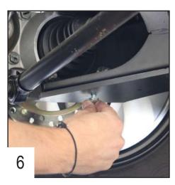
Use the TBHC 8x30mm screws + bolts and M8 washers to fix the guard on the back of the arm.
