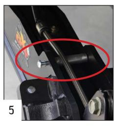
Make sure to place the middle spacer under the cable.
