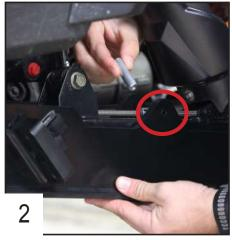
Place the allow spacer in the back hole.
