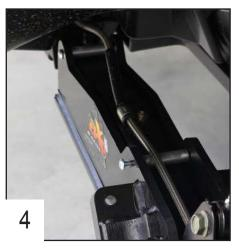
Place the 2 other alloy spacers in the holes and use the TBHC 6x20mm screws + M6 washersto maintain the spacers.
