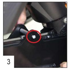
Use the TBHC 6x20mm screw + M6 washer to fix the spacer.
