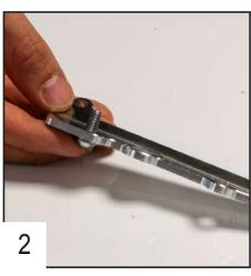
Place the TBHC 6x16mm screw on the 2 center holes of the longest aluminium part.
