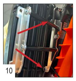
Place the 2 TBHC 6x16mm screws in the back holes without tightening them.
