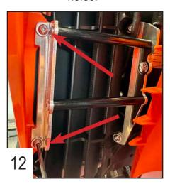
Place the TBHC 6x20mm in the 2 holes and tighten the four screws.
