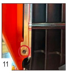
Put the plastic cover back on and place the plastic hole between the radiator and the guard.
