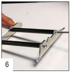
Tighten all the screws and repeat the operation on the other side.
