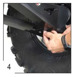
Place the TBHC 6x35mm screws + bolts and washers.
