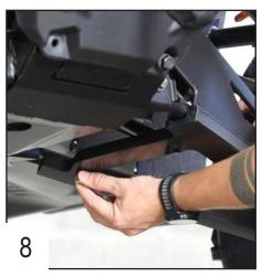
Use the TBHC 6x40mm screws, bolts and washers to fix the guard on the larger side.
