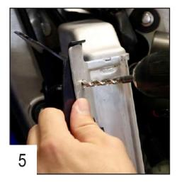
Use a 6,5mm bit drill and place the TBHC 6x16mm screw + EM6F bolt and washer.
