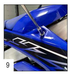
Place the OEM screw to finish fixing the plastic.
