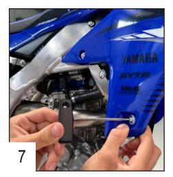
Place the TBHC 6x20mm screw + M6 washer in the bottom hole.
