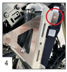
For a better fixation, you can drill a hole in the radiator and plastic.
