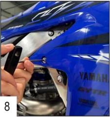
Place the TBHC 6x16mm screw + washer in the last hole.
