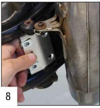
Place the front fixation on the frame. You can remove the exhaust for an easier assembly (only for the first time).
