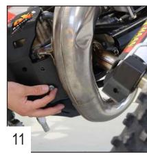
Fix the plate using the 2 special screws.
