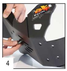
Fix the plastic block using a TFHC 6x30 screw + EM6F bolt and M6 washer then tighten.
