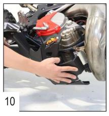
Insert the plate on the frame using the hook.
