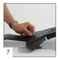
Place the TFHC 6x30 screw without tightening it.
