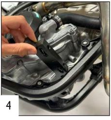
Place the front fixation on the frame.
