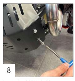
Insert the 2 THF 6x30 screws + alloy spacers and tighten.
