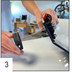
Place the smaller screw (6x25mm) in the bottom hole, the 6x30 screw on top and tighten.
