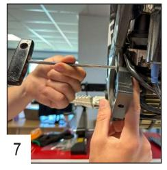
Place the front right fixation using 8x25 screw + EM8F bolt and tighten.
