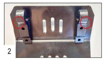
Place the rear hooks with the machined faces on the outside.
