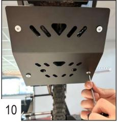
Lift the plate up and tighten the four 6x25 screws.
