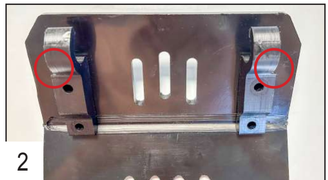
Place the rear hooks with the machined faces on the outside.
