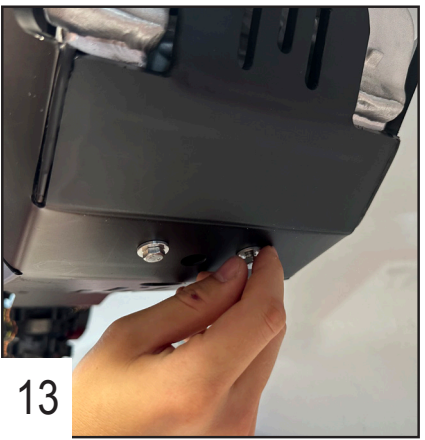
Place the TH 6x25 screws in the front holes.
