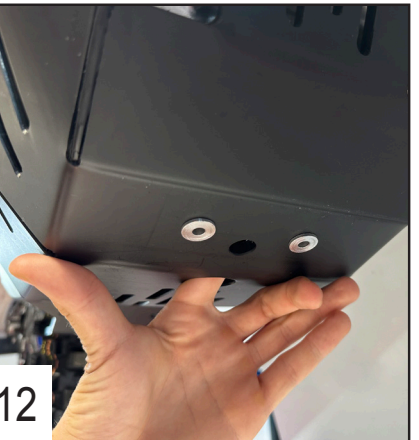
Use your finger to maintain the steel part in place and have the clamped bolts aligned to the holes.
