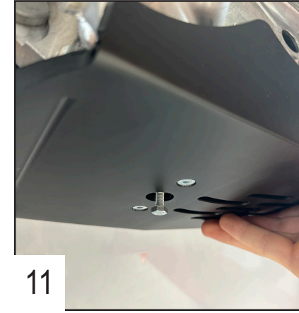
Place the TH 6x30 screw at the back first without tightening the screw.
