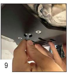
Place the TH 6x15 screw at the back first and tighten.
