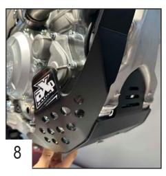
Place the plate, it must fit perfectly to the frame.
