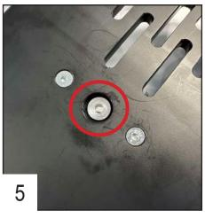
Place the alloy spacer on the back of the plate.
