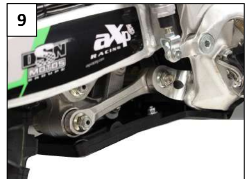
Plate N°41 + Tfhc 6x25mm + 2 M6 Washers + 2 Em6f
