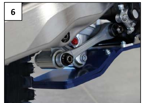
6 Put the rear plate Mettre la plaque arrière Tfhc 6x25mm + em6f + M6 Washers
